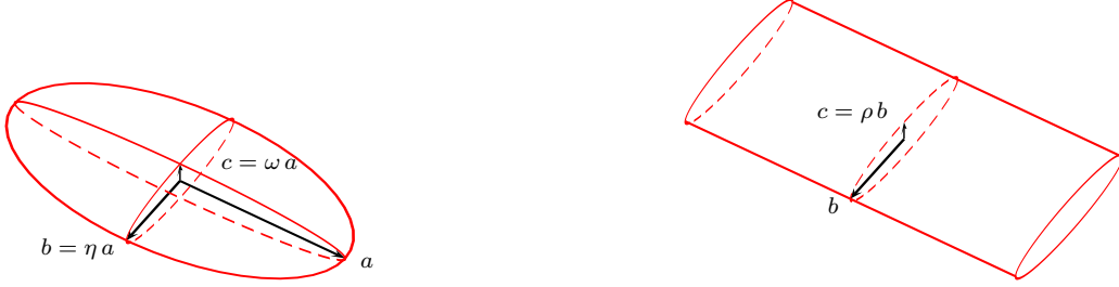
(a) Ellipsoidal crack
